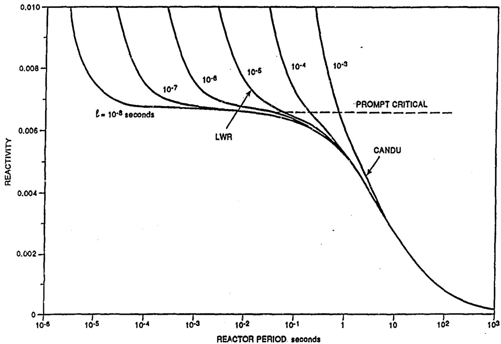
**Relationship Between Reactor Period and Reactivity for Various Neutron Generation Times**
